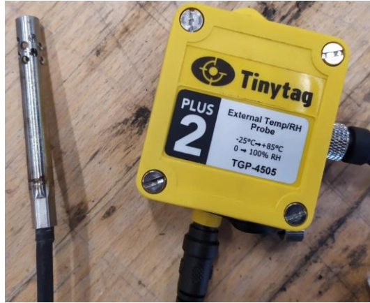
Figure 7. Tinytag Plus 2 (TGP-4505) with external temperature and RH probe.
